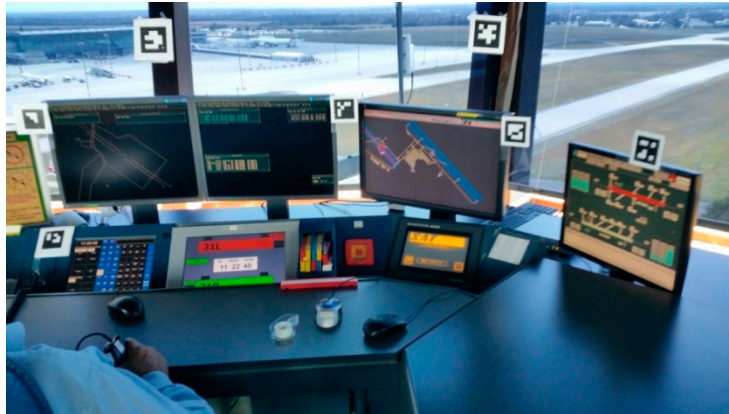
Fig. 3. The aerodrome controller position in the tower (the black and white markers are necessary for the automatic recognition of areas of interest)
